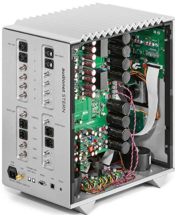
*The bottom section of the preamp houses no less than four 50 VA transformers which take care of either the positive or negative half cycles per channel. With a sieve capacitance of – for a preamp – awesome 176,000 microfarads they offer enough buffer capacitance to definitely feed every dynamic transient sequence in an unshakeable manner.*
