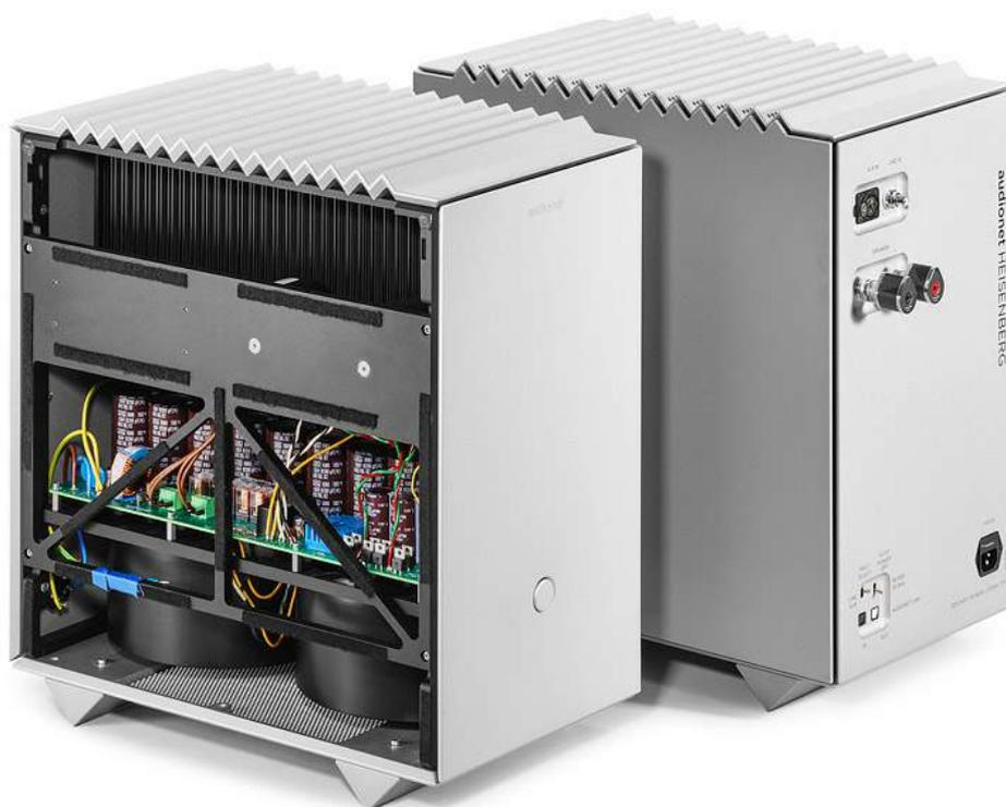
*Via the power switch on the front panel Heisenberg communicates its different operating conditions and also if it's generally well. Because if this isn't the case, the clear white one turns into a red LED ring which transmits its message through a morse signal code. Decoupled, encapsulated and in twin packs come the 1,200 VA transformers, whose energy is stored temporarily in a 200,000 microfarad buffer. 900 solid watts into four ohms are a true statement.*
